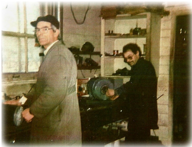
Andre and his son Denis repairing (rewiring) Electric motors
